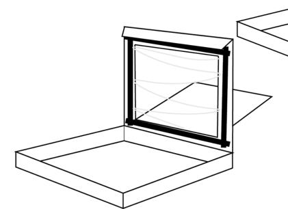
5. Tape clear plastic to the underside of the box lid to create a window under the flap.
